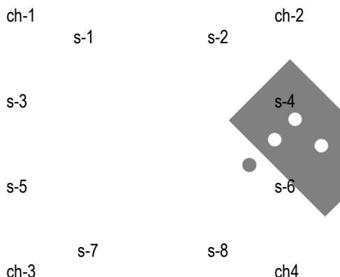
A stereo mix-down of the spatialised source is added to all channels to smooth discontinuities in the speaker set-up, room acoustics and audience location.
